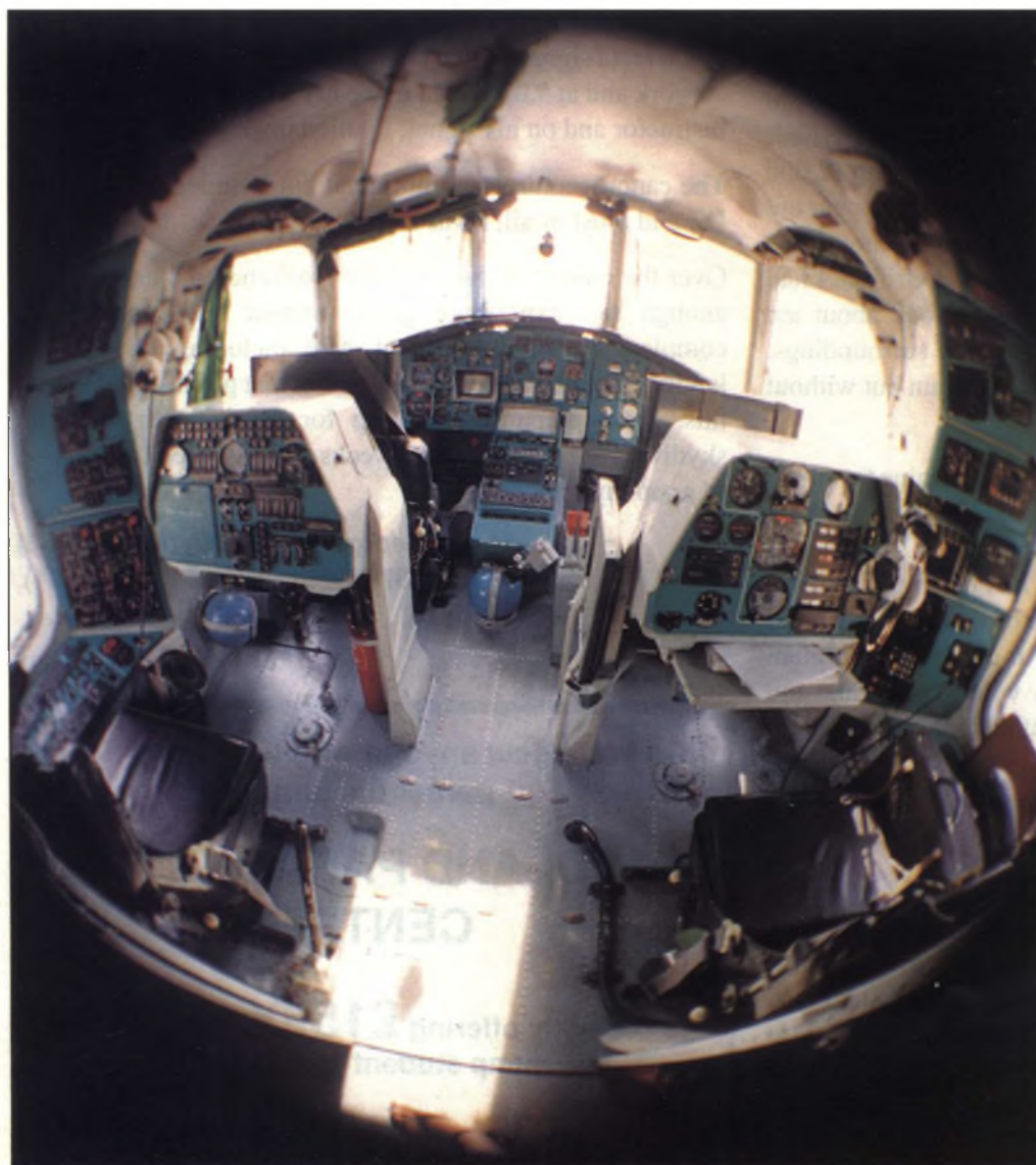
The flight deck for a crew of 4 plus Loadmaster on the MI-26
