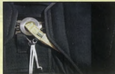
A special safety pin prevents premature container openings if release handles are accidentally pulled prior to drogue deployment
