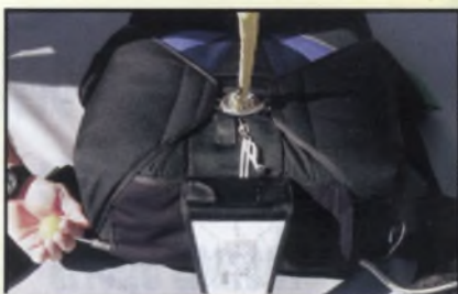
There are drogue release handles on both sides, left and right, either will open the container and release the drogue
