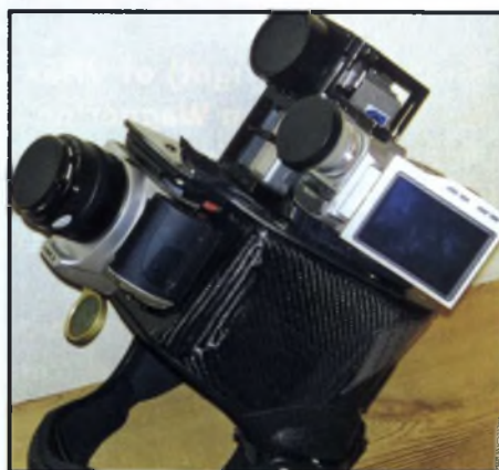
Brian's camera setup. Note the 3.5" LCD which offers teams a decent sized viewing screen on back to back loads. The two videos provide a back-up, one has an extra wide lens to ensure no grips move out of frame.
