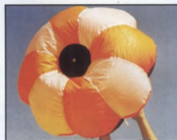
The Powershot is brightly coloured to assist finding it after a cutaway
