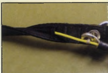
Twisted risers can grip the cutaway cable
