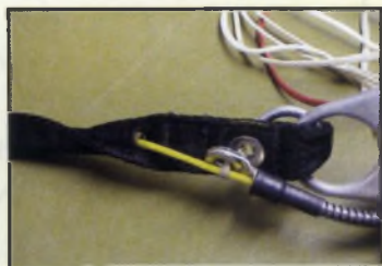
With hard riser channels, twisted risers no longer grip the cutaway cable
