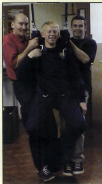
A 3 bloke test mimics a cutaway under a 3G force similar to a malfunction
