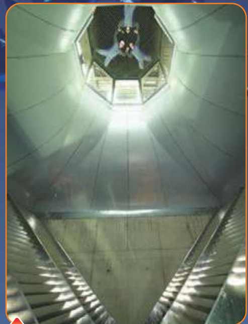
A view from deep within the plenum looking at the turning vanes (perfected by a NASA wind tunnel scientist) and up into the flight chamber where a three way is flying.
